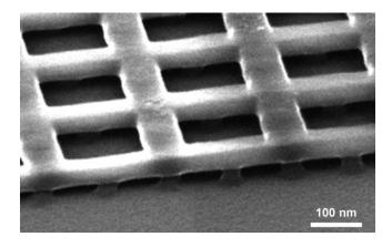
Figure 1. SEM image of a 3D supported cross grid structure from sample III fabricated by using the methods described in this paper (tilt angle of 55°). Freestanding top layer was patterned in HSQ and supporting bottom layer was patterned in PMMA. The two layers were exposed in a single electron-beam writing step without intermediate alignment of the pattern.
