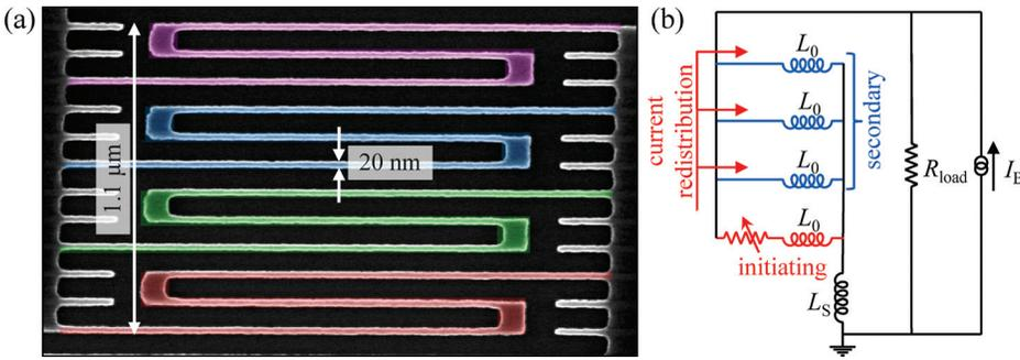
FIG. 1. (a) Colorized scanning electron microscope (SEM) image of a 4-SNAP resist (hydrogen silsesquioxane) mask on NbN with each section colored differently. (b) Equivalent electrical circuit of a 4-SNAP. The arrows pointing at the secondary sections represent the current redistributed from the initiating section to the secondary sections after the initiating section switches to the normal state.
