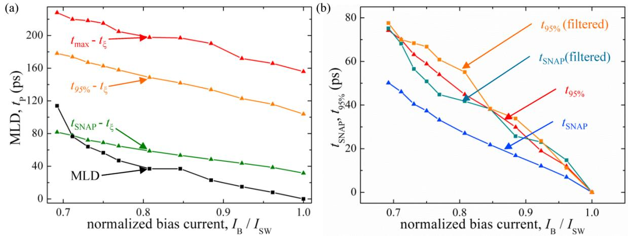
**Figure SM 3. a.** Experimental MLD vs  $I_B$  (black squares) and simulated  $t_p$  vs  $I_B$  (red, orange and green triangles) for the 2-SNAP of Figure 2b. The values of  $t_p$  were calculated by using different thresholds on the SNAP pulse as references:  $t_{\max}$  (red curve);  $t_{95\%}$  (orange curve); and  $t_{\text{SNAP}}$  (green curve). **b.**  $t_{95\%}$  and  $t_{\text{SNAP}}$  of the pulses shown in Figure 3a (triangles) and of the filtered pulses vs  $I_B$  (squares).
