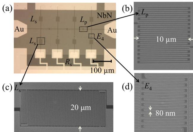
FIG. 3. Images of a four-element array. (a) Optical micrograph of the array. (b) SEM image of the current-splitting inductor  $L_p$ . (c) SEM image of the inductor  $L_s$ . (d) SEM image of a SNSPD from one of the pixels with an active area of  $2.6 \mu\text{m} \times 3.0 \mu\text{m}$ .
