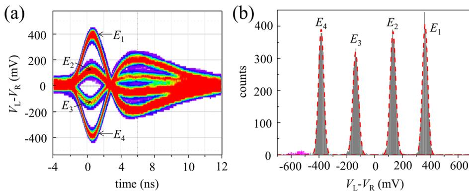
FIG. 4. Position discrimination of detection events in the four-element array. (a) Persistence map of  $V_L - V_R$  captured by the oscilloscope showing pulses originating from  $E_1$ ,  $E_2$ ,  $E_3$ , and  $E_4$ . (b) The histogram of  $V_L - V_R$  sampling for 15,160 pulses with a 5 mV bin size. Peaks are fit using Gaussian functions (dashed-red lines). The counts outside the four peaks (purple coloring) were possibly from multiple-count events.
