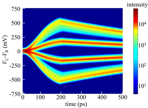
FIG. 2. Monte-Carlo electrothermal modeling of the differential signal  $V_L - V_R$  in the four-element array, including circuit variations. The pulses from top to bottom are the single-element triggering cases occurring at  $E_1$ ,  $E_2$ ,  $E_3$ , and  $E_4$ , respectively. The color of the pulses shows the intensity of the position where the traces appear.
